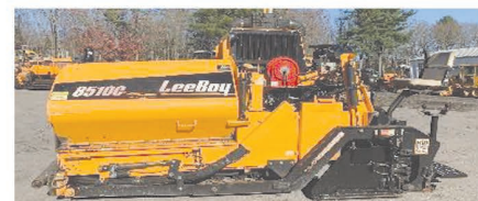
2017 LeeBoy 8616 Kubota 111 HP Diesel Engine with 8-15' Legend Electric Screed. 9 Ton Conveyor Hopper and Poly Pads. SLOPING SCREED EXTENSIONS HEATED ENDGATES Power Crown $110,000
