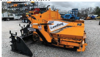
2015 LeeBoy 1000 Kubota 44HP Diesel With 8-13' Legend Propane Screed. 5.5 Ton Dump Hopper and Steel $57,000
