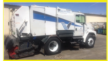
2002 Elgin Broom Bear Freightliner FL70 CAT 3126. 122,773 miles and is fully operational. Mechanical sweeper with rear rotary and 2 gutter brooms. Large water tank. $22,500 Sean 559-647-0462 to discuss purchase and transport. (x/C-20)
