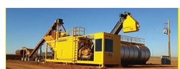
NEW 40 TPH Asphalt Plant & AC tank 400K , Counter flow, External Mix, Baghouse with fines recovery system, Rap Collar, Call 305-436-8228 or 754-235-8228 (Financing Available) admin@dmiasphalthequipment.com (x/A-21)
