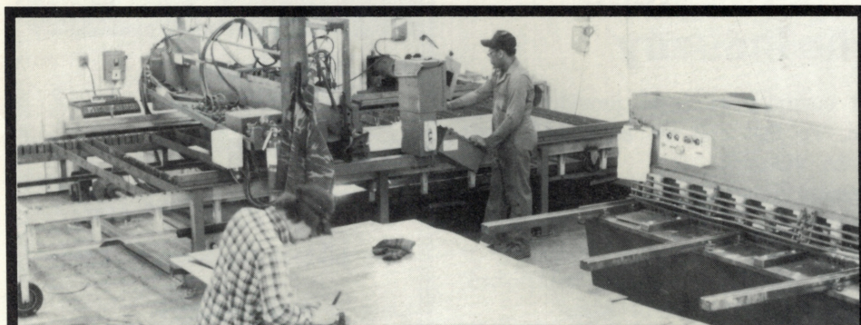
Here is our automatic plasma burner used for fabrication of steel plate. Pictured are two of our qualified burner operators. In the foreground Johnny Barnes is measuring steel prior to cutting, while Bob Brandon cuts a piece of stock to dimension.
