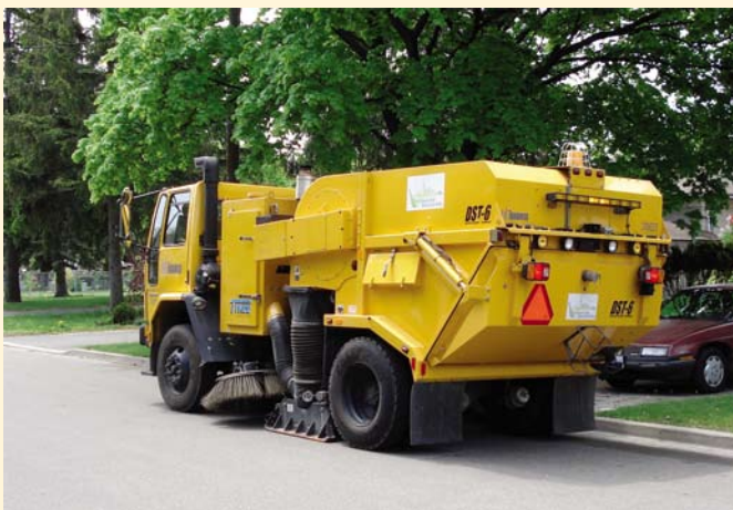
Figure 2: A City of Toronto “dustless” regenerative air sweeper on display
