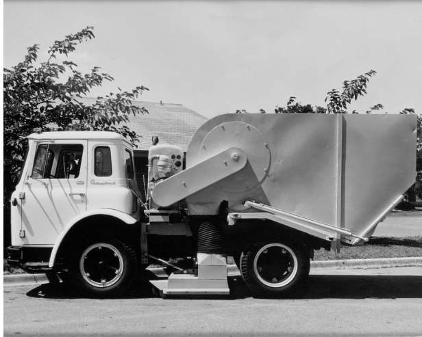
Original Young “Air-Flo” Truck Mounted Regenerative Air Sweeper – circa 1966
