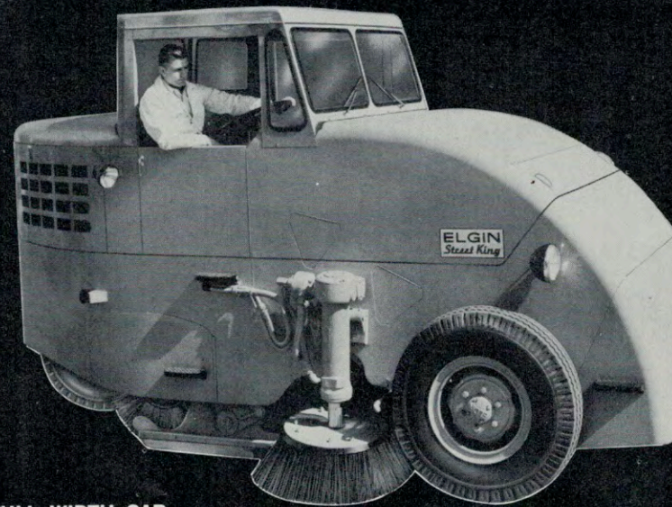
FULL WIDTH CAB Full width, heavy gauge steel cab features shatterproof glass windshield and rear windows. Comes equipped with dual electric windshield wipers and available with either side curtains or full door with roll down windows.
