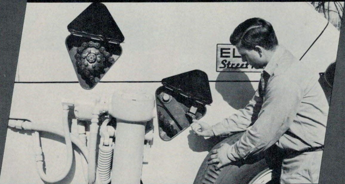
Special panels provide access to the main drive chains and chain tighteners.
