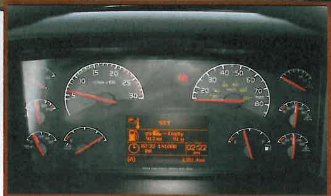
The Volvo dash has two liquid gauges flanking the driver display. On the right side is fuel; the left side is for the diesel exhaust fluid, or DEF.
