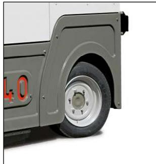
CS140 "TwinAction" has an integral steering system on all 4 wheels with symmetrical front and rear angles (the same centre of rotation for the two axles) and turning circle of 4,25 m. Together with great manoeuvrability, even near walls or fences, and guarantee the necessary ease of handling to operate in places where the space is limited such as historical town centres or cluttered areas, at the same time guaranteeing maximum vehicle stability during transfer even at the highest speed.
