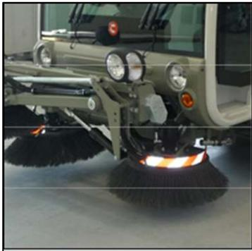
The "TwinAction" street sweeper is equipped as standard with one Right side brush, whilst the Left and Translating ones are optional. In fact the new design of dust collection system, allows to reduce the use of side and translating brushes, to convey the dirt from the edges (curbs or walls) to the central area only, where the main brush works.
