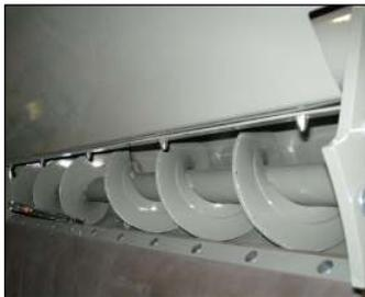
The screw conveyors consist of two steel shafts, both equipped with a spiral which, hydraulically moved, rotate on the same axis, conveying dirt and debris of different dimensions close to the suction outlet.
