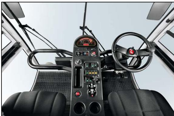
The cabin is comfortable because it is spacious and insulated with anti-vibration supports. It is comfortable to drive and the large windscreen provides maximum external visibility for the operator, making manoeuvring and control over the collection are easier. The activation commands, simple and intuitive are grouped on a central console. The others are on the front part of the roof, both easily accessible from the working position. On request the machine can be customized with climate control
