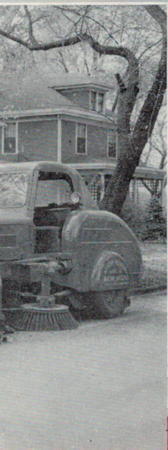
The Leaf Broom attachment handles bulky accumulations of leaves quickly and efficiently while in no way interfering with regular sweeping. Spring suspension mounting allows the broom to follow contour of street.
